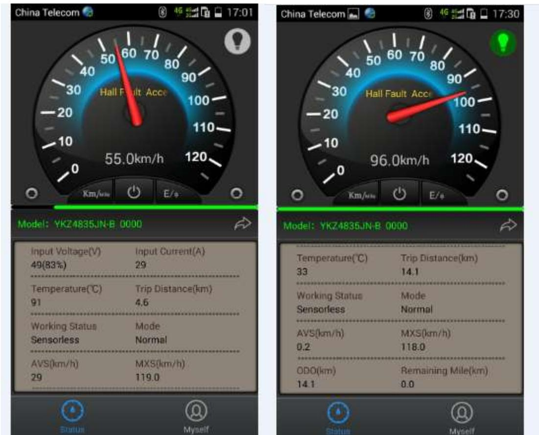
This is the working status interface of YUYANGKING controllers, which can display various working statuses of controllers.
