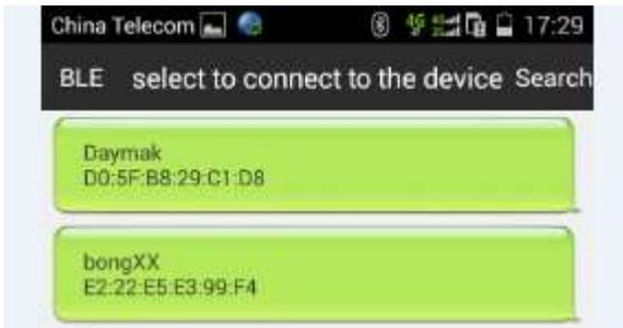
Connect the device, it will show connecting, wait until show to enter password(It takes 20-40 seconds first time). Enter password 1234, then log out the App and log into again, it will show the Bluetooth name.
